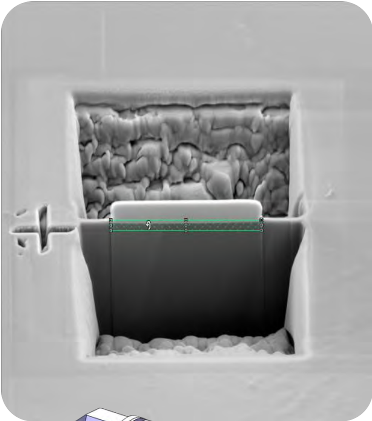
Pillars for mechanical testing
